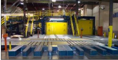
Multiple fork truck stations are an option for load sorting or simply to increase the number of units to load or unload at one time.
