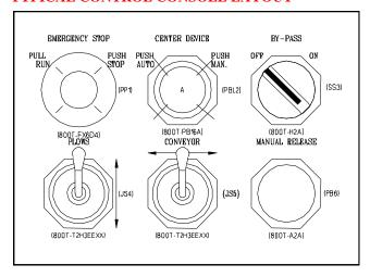
This typical control console (*Above*) is used as a manual override control station. Located on the operator side of the device for easy access it contains both emergency stop and manual override controls.
