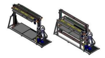
Conveyor beds open / close using linear actuators driven by servo motors.
