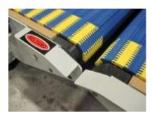
(Left) Detail of a typical Stedi-Stak platform. The tight turnaround of the chain reduces the gap between conveyors to a minimum. (Right) Gear motor directly coupled to the drive shaft using a key way.
