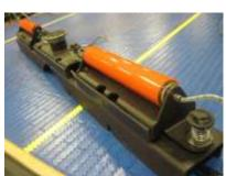
Left) Detail of a typical Stedi-Stak platform. The tight turnaround of the chain reduces the gap between conveyors to a minimum. (Right) The chain wraps around equidistantly-spaced sprockets along the drive shaft.
